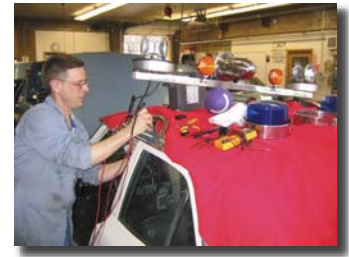
Tom Leahy of Seattle's DIT installing the car's "Twin Beacon Ray" light bar
