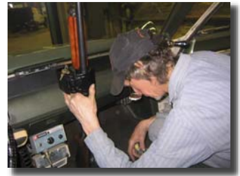
Paul Kozelisky from Seattle's DOT Metal Shop making the shotgun lock bracket
